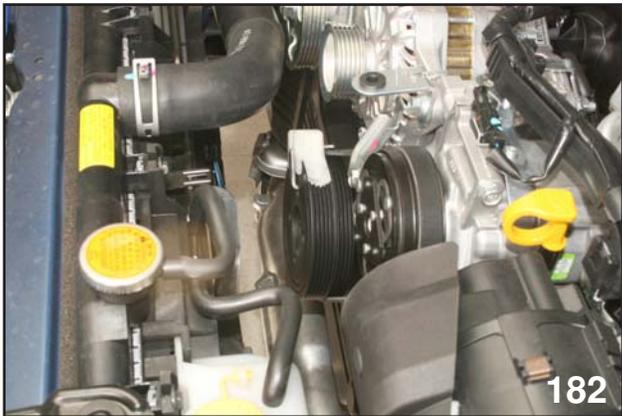
*Belt Fully Engaged on Crankshaft Pulley*
