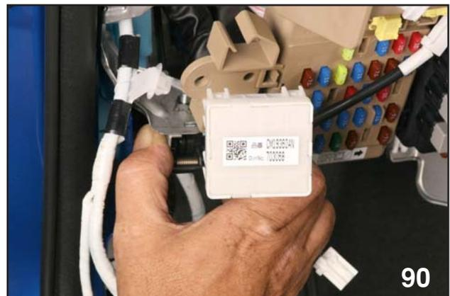
*Releasing Multi Joint Connector*
