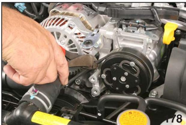
*Cutting off Air Conditioning Compressor Belt*
