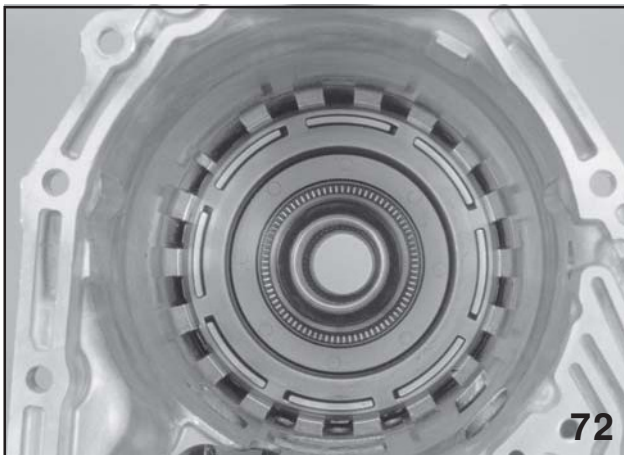
Reverse Brake Piston Snap Ring In
