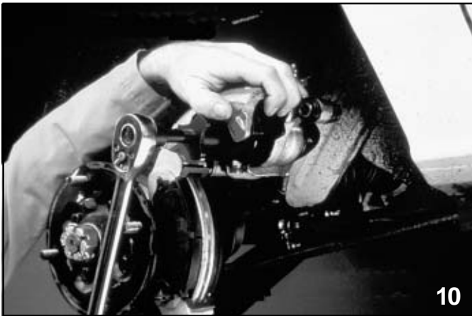
Depressing caliper piston (older)
