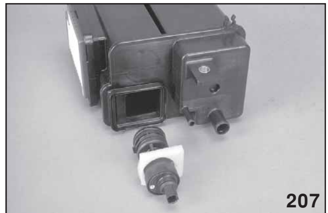
Drain Valve Separated from Canister (NOT SERVICEABLE)
