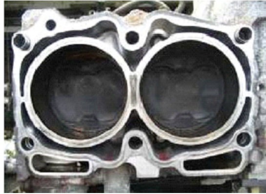
Finished cleaning (block)
