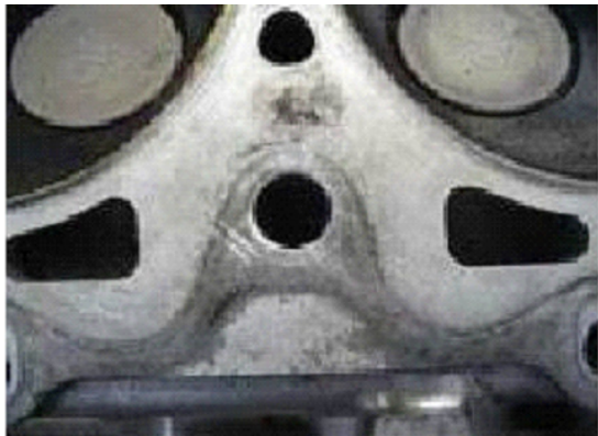
After cleaning coolant sealing portion (head)
