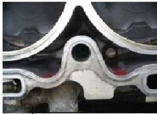
After cleaning coolant sealing portion (block)
