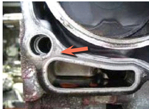
Rubber coating residue on oil sealing portion
