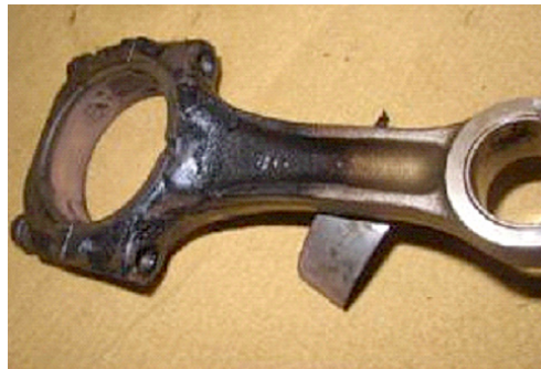
Rod Bearing Spun from Lack of Oil
