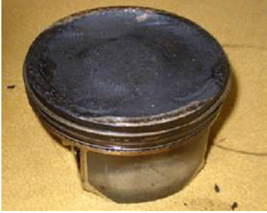
Ring Land Damage from Detonation
