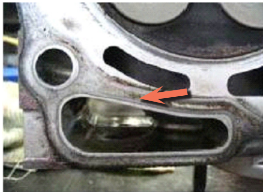
Rubber coating residue on oil sealing portion
